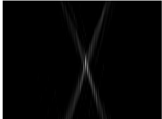
Figure 6. Focal point beam profile mapped by Schlieren system
